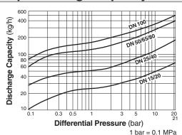
Note: 1. The discharge capacity is the maximum continuous condensate discharge 6 °C below saturated steam temperature.
